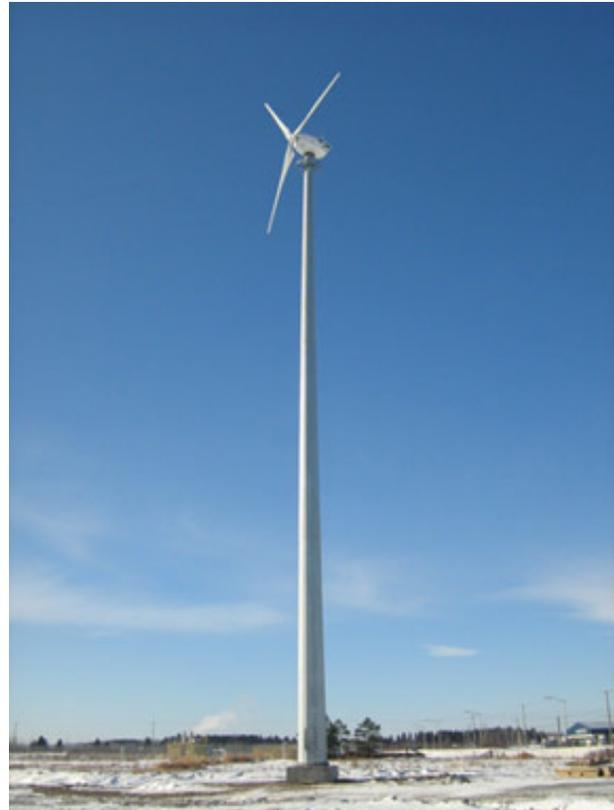
Tower options include free-standing and tilt monopole and free-standing lattice. Available hub heights are 18, 24, 30, 36, and 42 meters. Eocycle notes that all tower are hot-dip galvanized and are supplied with work platform, climbing step bolts ad safety cable. Standard warranty is two years; extended warranty is five years. The turbine can be equipped for arctic temperatures.
