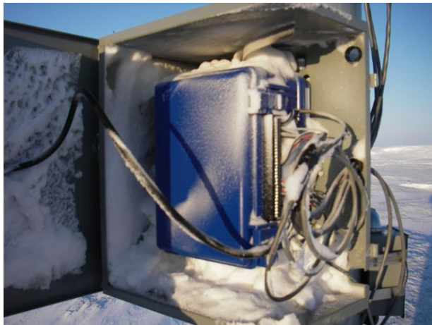
Datalogger with snow in weather box; D. Vaught photo
