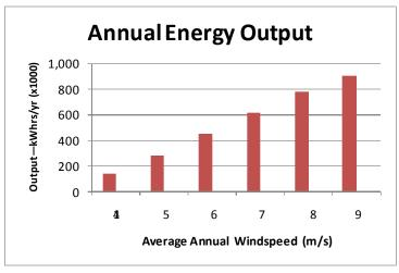
The Power and Energy Curves shown are valid for 1.225kg/m3 air density, clean blades and undisturbed horizontal air flow. In the stall range, at wind speeds over 16 m/s, the power factor may deviate from that shown. For the Energy Graph, a Rayleigh wind speed distribution and 100% availability is assumed.
