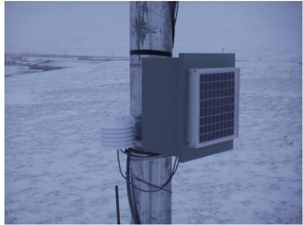
Datalogger weather box and PV panel; D. Vaught photo
