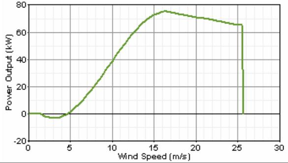
**Northwind 100/20:** 100 kW rated power output, 20 meter rotor (19 meter rotor blades with 0.6 meter blade root extensions added), stall-controlled (power curve provided by Northern Power Systems). Available tower heights: 25 and 32 meters. Additional information is available at <http://www.northernpower.com/>.
