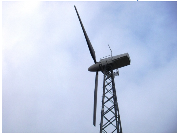
Vestas V19 wind turbine (similar V17 turbine in Kokhanok shown below)
